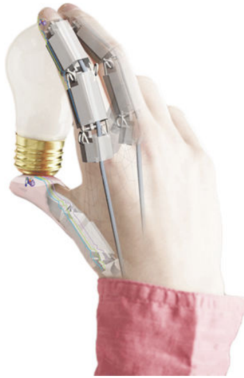
Figure 2: Mesofluidic prosthetic fingers with FILMskin patch.
